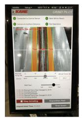
As engineers capture more and more visual data for different types of weld seams, they teach the GRIT Vision System to grind seams on various-sized tank shells and parts. Over time, the cobot solution learns to detect variations in welds and improve its accuracy.
