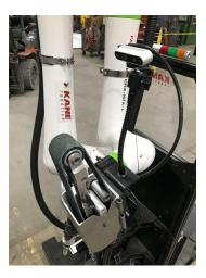
direct the weld-grinding tool along the correct path. The intelligent system learns to "see" the varying weld seam even as it disappears, as it has been taught to differentiate between an unfinished weld and a finished weld.
