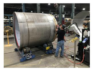
In 2023, the company was seeking a more sustainable method for weld grinding. Kane Robotics offered its mobile, low-cost and versatile <u>GRIT<sup>IM</sup> cobot</u> that combines a robotic arm with a variety of end-of-arm tools that are preprogrammed to perform various types of material removal tasks, including metal grinding.
