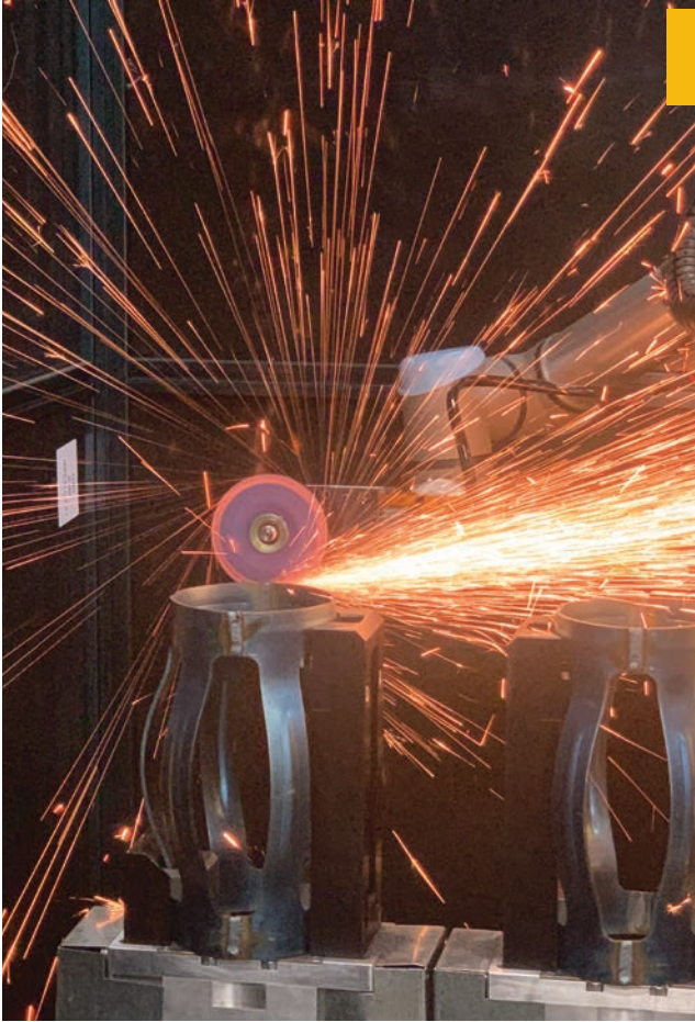
Fig. 2 — End-of-arm tools on a robotic arm grind welds and help human technicians avoid hazards.
