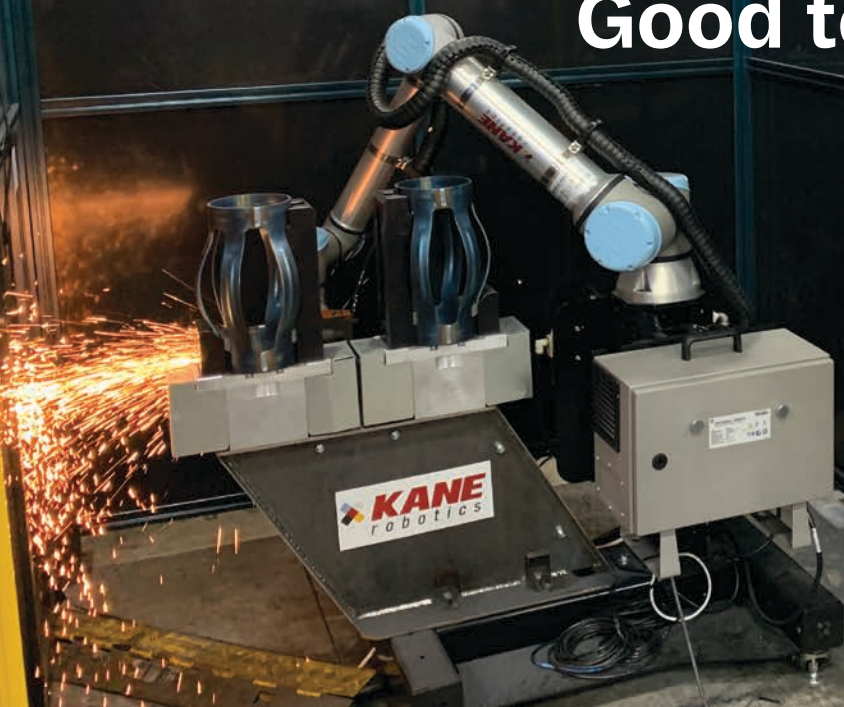
Fig. 1 — An operator looks on as Kane Robotics' GRIT™ ST grinds centralizers for oil and gas application.
